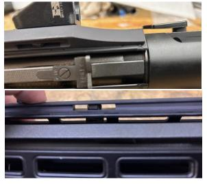
Using the supplied wrench, turn the hex head screws clockwise. Make sure the M-Lok nuts rotate a full 90 Deg. so they are perpendicular to the rib. Once the nut has rotated to the correct orientation, snug the screw down fully.
