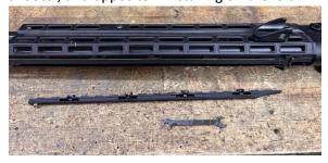
The M-Lok nuts are typically snugged up against the bottom of the rib for shipping. It is recommended to back them off at least .100" from the bottom face of the rib, or about flush with the bottom of the screw. The long edge of the nut should be parallel with the Rib.
